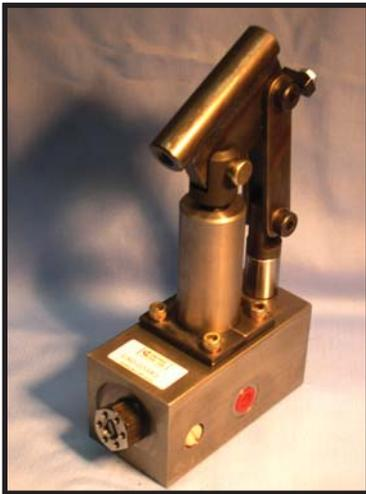
The modified pump shown on the left was designed to meet challenging specifications for a customer that required a custom adjustable operating handle interface, non-standard port sizes and a special design for the release screw. We are able to incorporate all of the customer requirements into the final unit so that no field modifications are needed. This saves OEM and user customers both time and money.
