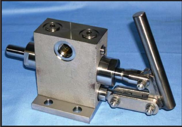
The pump shown on the left is a custom built all Stainless Steel, double acting unit built for use on offshore equipment in a marine environment as the emergency power source used to open or close watertight passage doors. This pump features a displacement of over 4 cubic inches per complete stroke and is rated for 1000PSI service. Oversize internal passages and ports allow for maximum fluid displacement in an application where output flow is critical.
